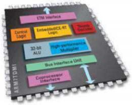
The ARM7TDMI has a core based on the fourth version of the ARM architecture. This implementation uses a three stage pipeline - a standard fetch-decode-execute organization.
